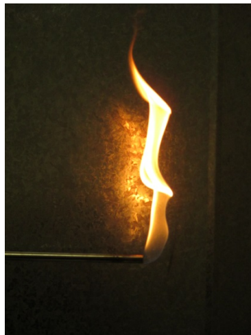
Figure 3. Photo of a Tube Burner showing a 240 mm flame:
