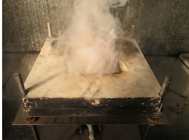
Figure 7. 9 seconds after ignition (a failing barrier)
