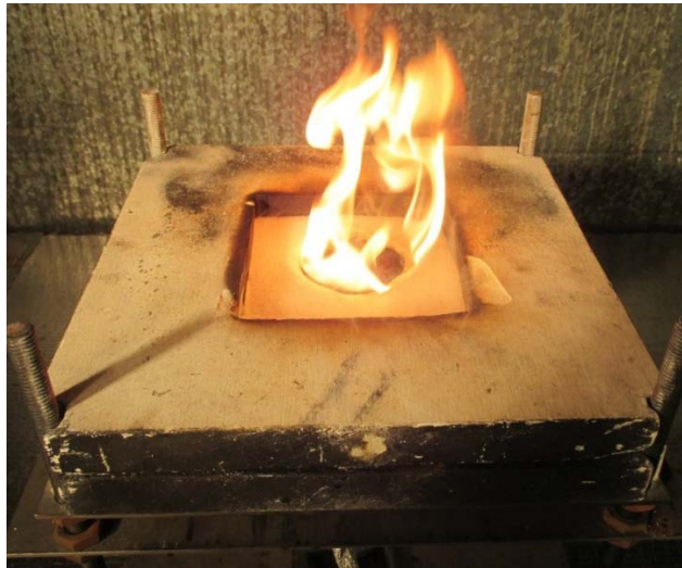
Figure 8. 12 seconds after ignition (a failing barrier)
