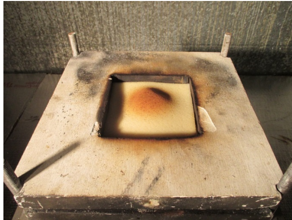
Figure 5 Top shot, 50 seconds ignition (a passing barrier)
